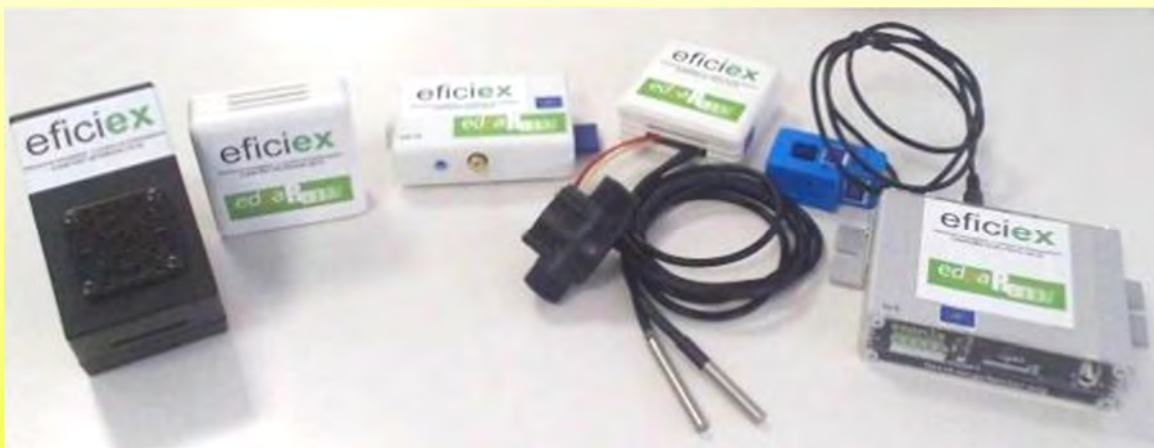
EFICIEX sensor system. From left to right: (1) Indoor comfort sensor, (2) Outdoor comfort sensor, (3) Base station (Raspberry Pi®), (4) water and gas consumption sensor and (5) power consumption sensor.
