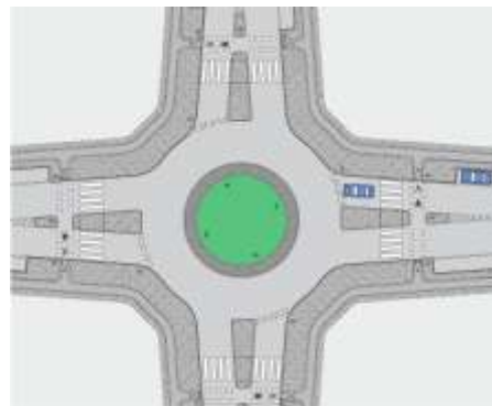
Single-lane roundabout with cycle track, without right-of way for cyclists. Notice the more angular design.
