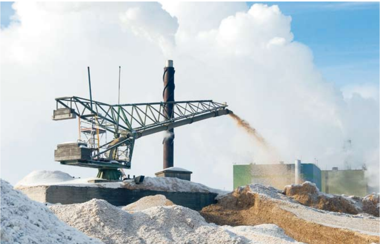
Wood chips are used as a raw material for the chemical pulp and bark is incinerated for energy in the power plant.
