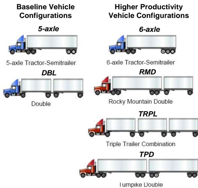
**Figure 8: Vehicle configurations considered in the ATRI study [ATRI, 2008]**
