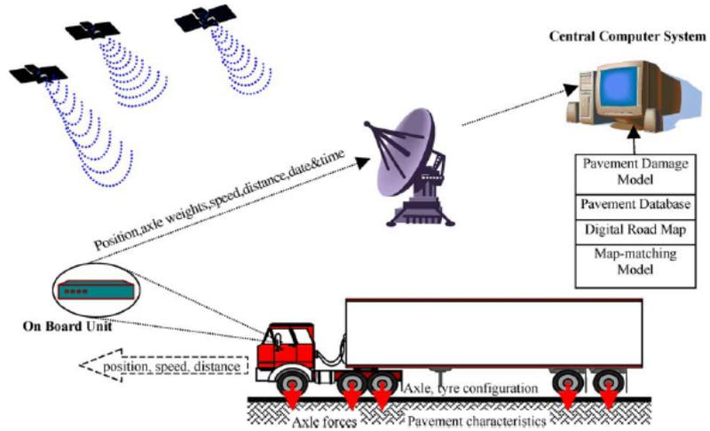
Figure 19: Overview of the pavement damage allocation system described by [Dodoo and Thorpe, 2005]
