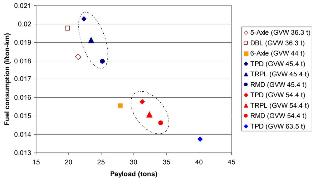
**Figure 9: Specific fuel consumption vs. payload for the different vehicle configurations**
