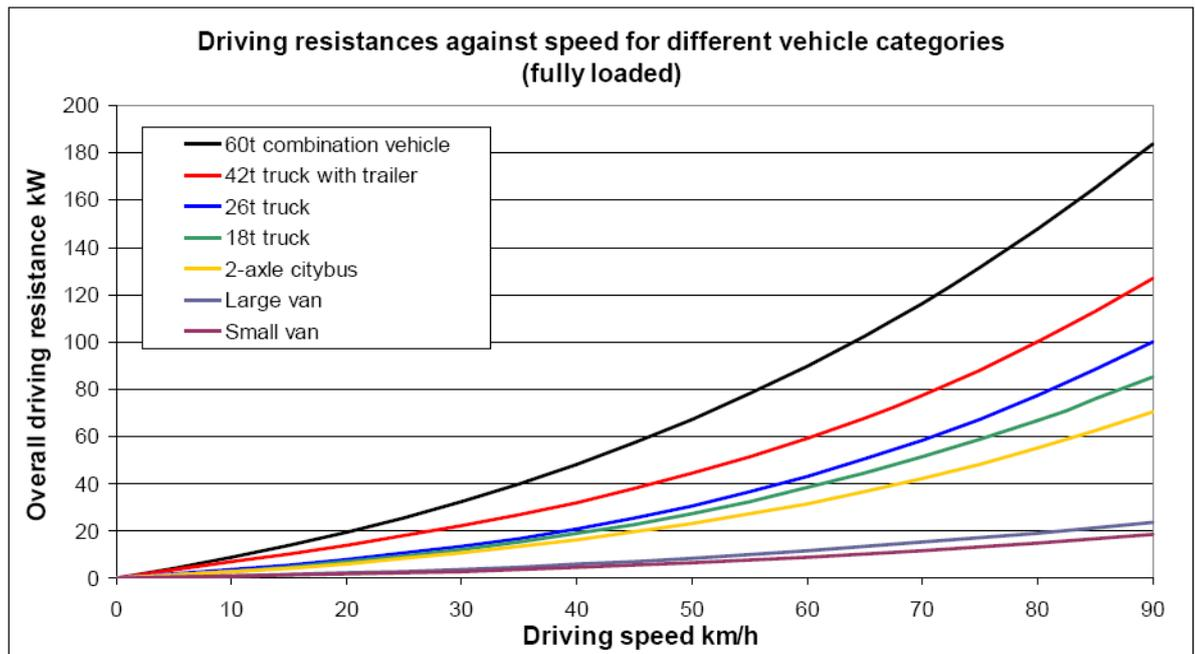
**Figure 11: Power needed to overcome the tractive resistance vs. speed**
