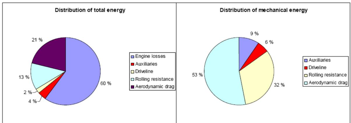
**Figure 2: Relative distribution of energy for a semi-trailer combination (at constant speed of 104 km/h)**
