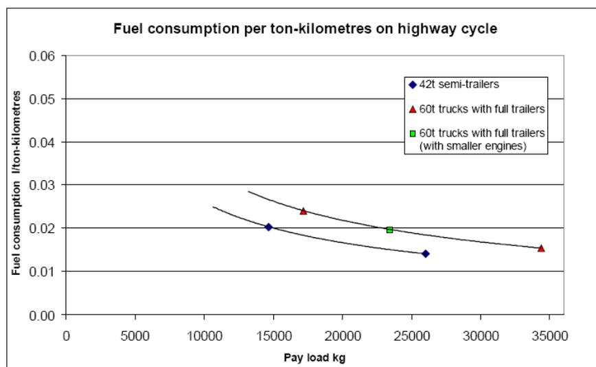
**Figure 7: Influence of payload on specific fuel consumption**
