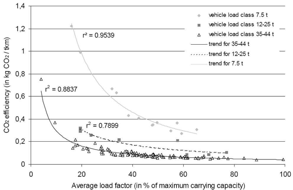
**Figure 6: CO<sub>2</sub> efficiency in relation to load capacity utilisation and vehicle size class**
