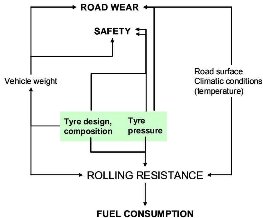
Figure 15: Schematic view of the effects of tyres on energy, safety and road wear (vehicle speed is not considered)
