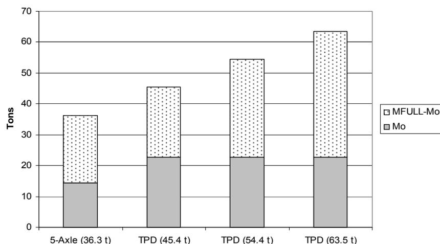
**Figure 10: Differences in tare weight and payload between the TPD and the baseline 5-axle vehicle**
