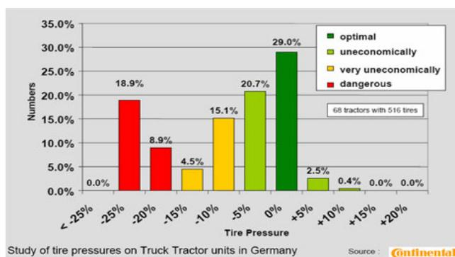
Figure 16: Tyre pressure on truck tractor units in Germany (from Continental)
