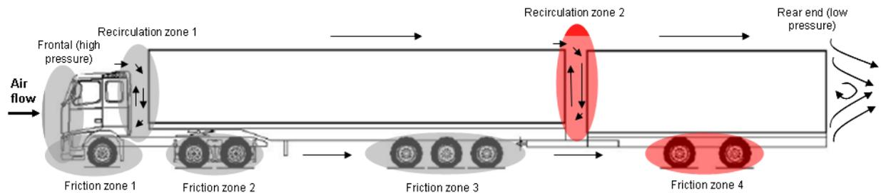
**Figure 12: Illustration of additional drag sources for LHVs (e.g. tractor, semitrailer and centre-axle trailer)**
