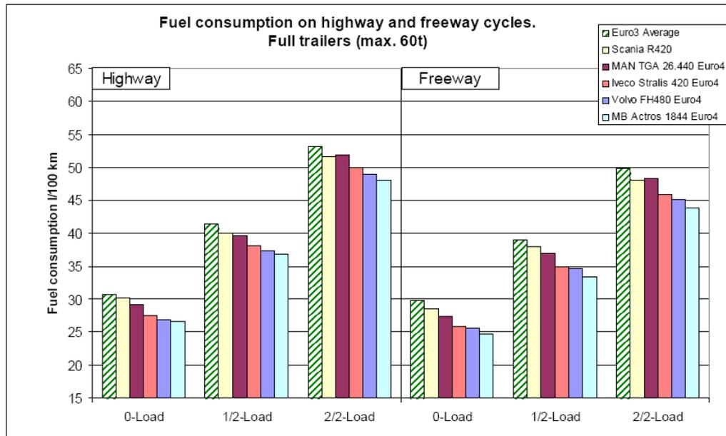
**Figure 4: Influence of payload on fuel consumption for 60t LHV's (type approval measurements)**
