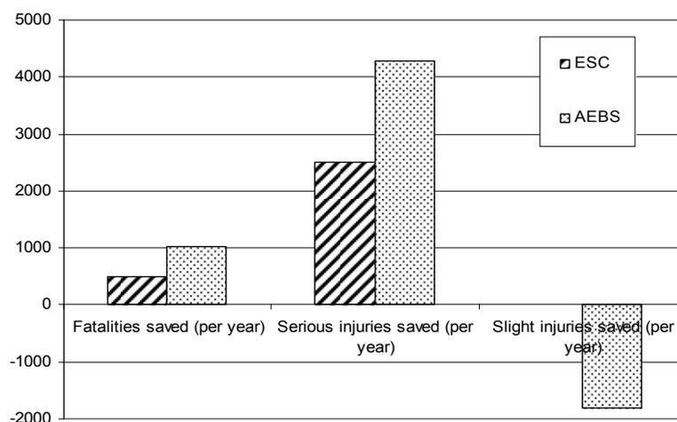
**Figure 18: Effect of ESC and AEB systems on safety for heavy vehicles**
