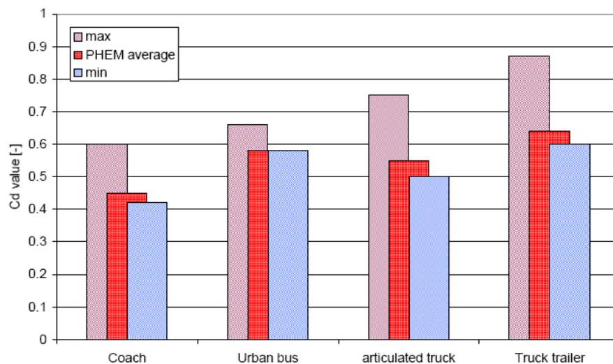
**Figure 13: Range of aerodynamic drag coefficients of different HDVs**
