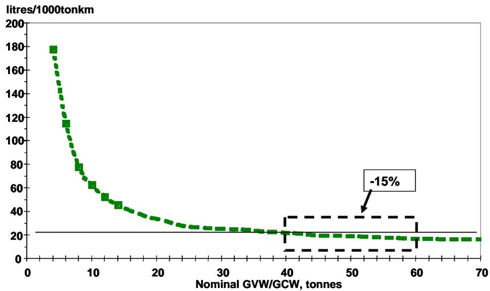
**Figure 5: Specific fuel consumption vs. Gross Combination Weight (i.e. total vehicle weight)**
