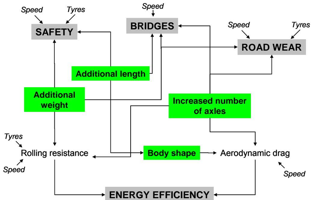
**Figure 1: Schematic overview of effects associated with LHVs on energy, infrastructure and safety**
