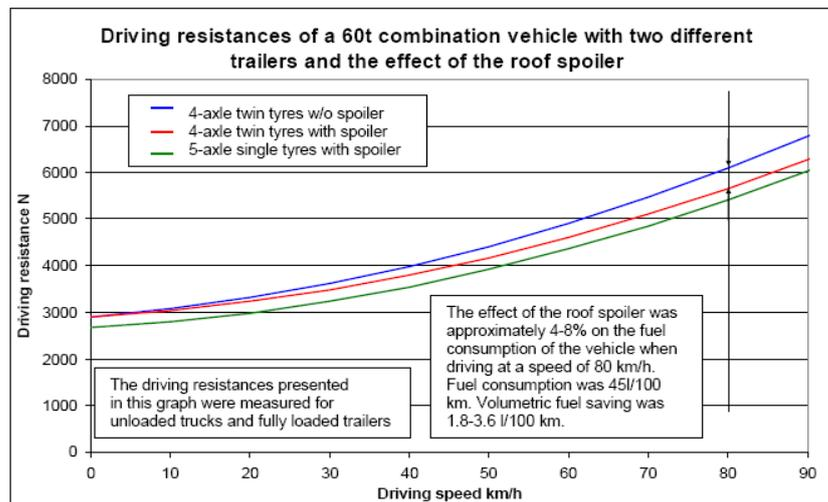
Figure 14: The air deflector's –and different trailer type's effect on the tractive resistance
