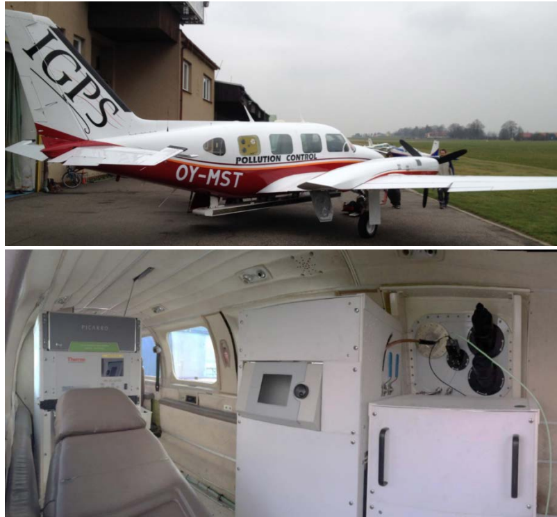
Figure 3. The ship surveillance system installed in a Danish Navajo Piper aircraft (OY-MST) (upper). To the left the gas rack is shown, in the middle the particle rack (Not applicable here) and on the right side the optical rack. In the upper right part of the picture a probe plate is shown containing telescopes and sondes.
