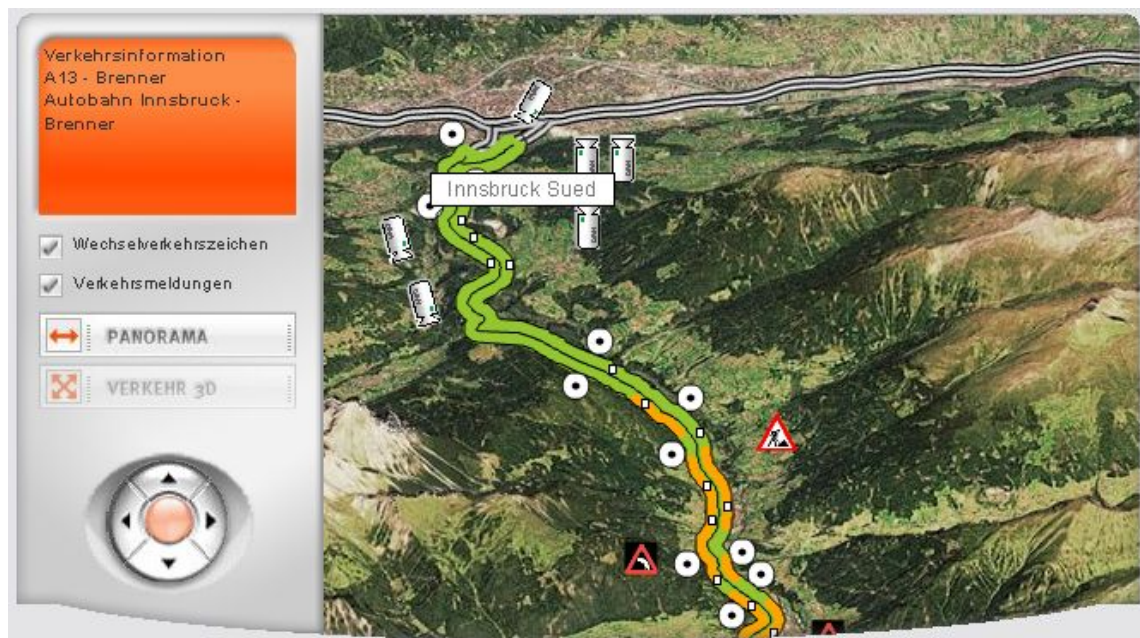
Figure 16-9: Road Pilot 2: Dynamic traffic information tool incl. traffic notes (red box on the left) for the motorway between Innsbruck and the Brenner (3-dimensional). The colours indicate the traffic situation. Green: free-flow, yellow/orange: dense traffic, red: congestion. Source: www.asfinag.at (30.08.06, 4 pm)
