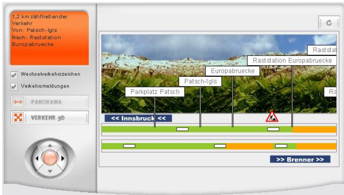
Figure 16-8: Road Pilot 2: Dynamic traffic information tool incl. traffic notes (red box on the left) for the motorway between Innsbruck and the Brenner (panorama view). The colours indicate the traffic situation. Green: free-flow, yellow: dense traffic, red: congestion. Source: www.asfinag.at (30.08.06, 4 pm)
