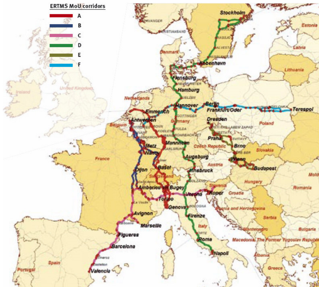
Figure 6.3 The six corridors on which the EU and national railways have agreed to deploy ERTMS
