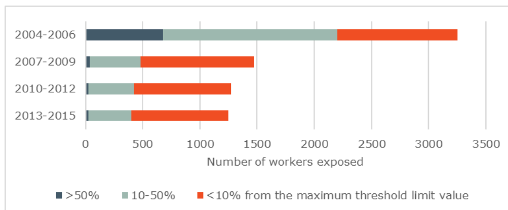
Figure 4.2. Trend in exposure to asbestos during 2004-2015. The threshold value (OEL) used in all calculations is 0.1 \text{ fibres/cm}^3 (Exposure database FINJEM of the Finnish Institute of Occupational Health, version 2016, FIOH 2020a).
