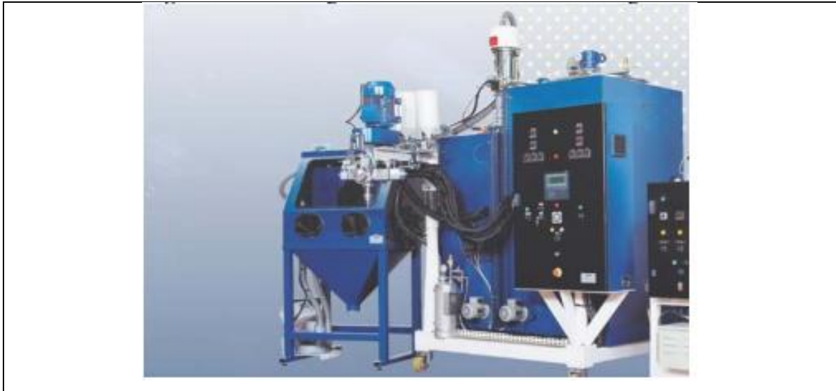
Figure 3.3: Glove box and automated moulding machine used in polyurethane moulding Reproduced with courtesy of REACHLaw
