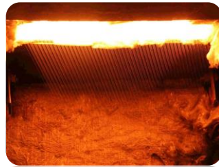
Basalt stone melting on 1400 degrees
