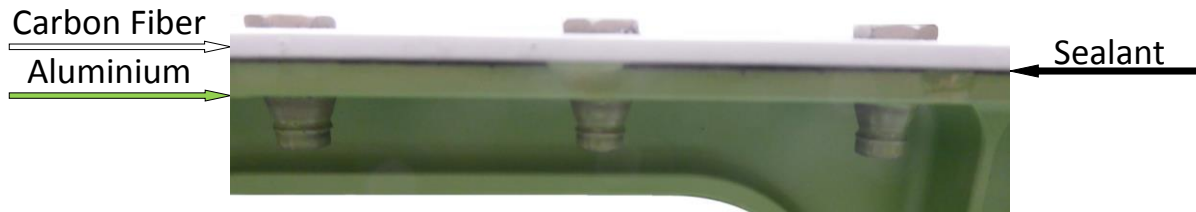
Figure 1. Typical assembly where one way assembly and automated fastening would be preferred
