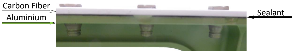
Figure 1. Typical assembly where orbital drilling could offer substantial benefits over traditional drilling methods
