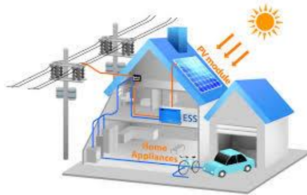
Figure 17 - The Prosumer concept. The Power transmission lines turn from one-way to two-way ones
