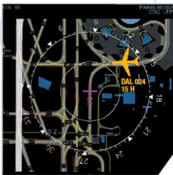
Example of Navigation Display. Position and trajectory of other aircraft on taxiways are
