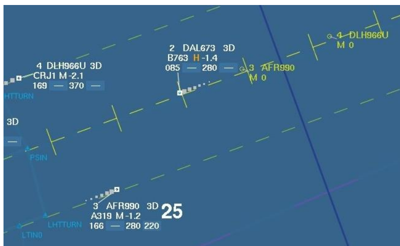
FAGI radar display with a/c DLH996U and AFR990 on downwind segments and their
