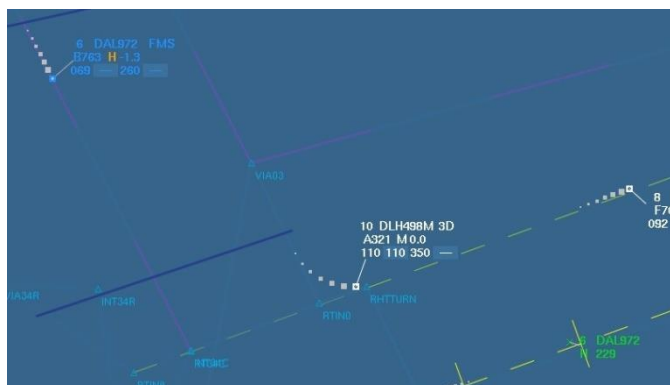
FAGI radar display with equipped a/c DAL972 and its (green) ghost on the centreline
