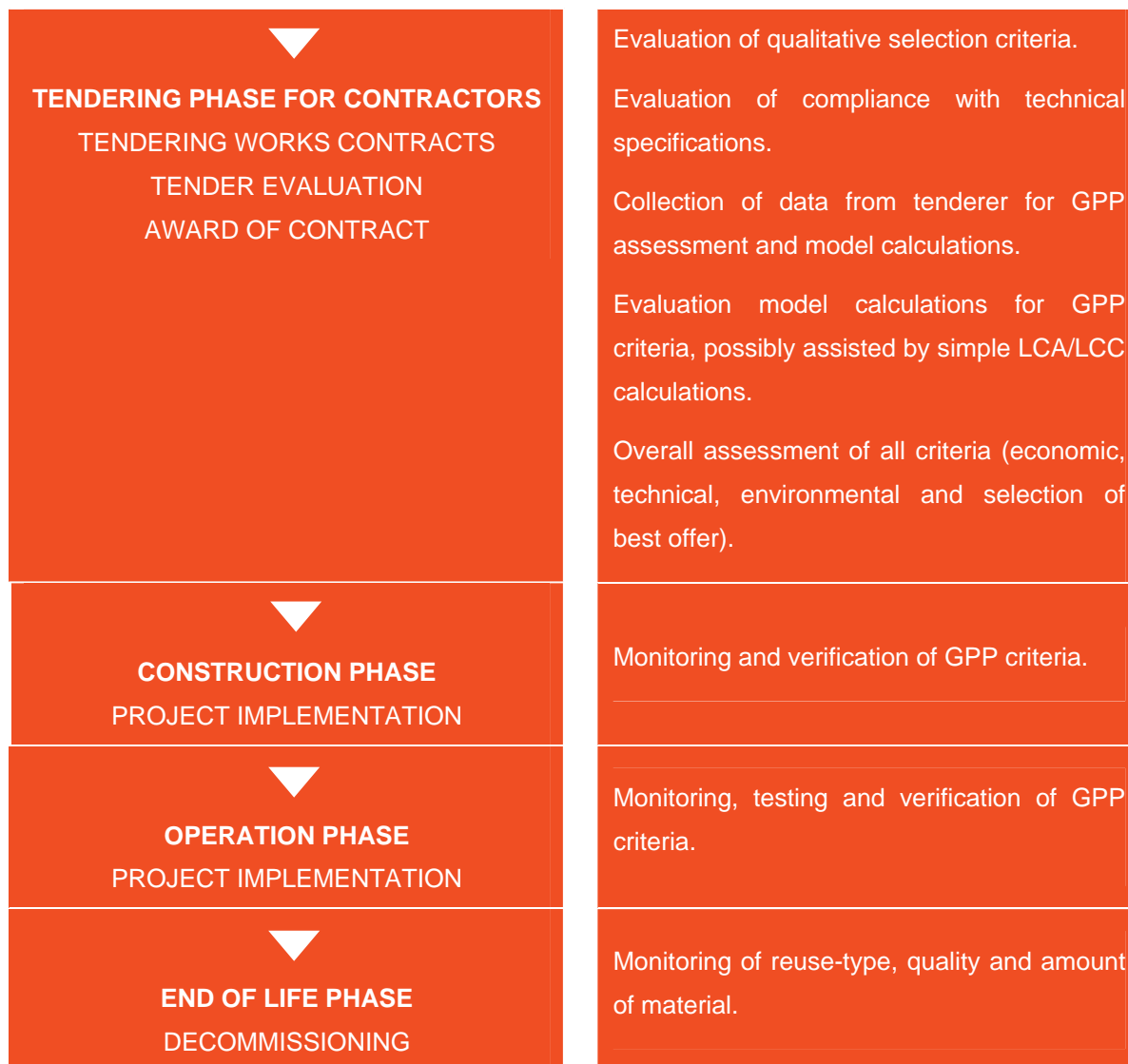
Figure 4-1 Project development and how to use GPP criteria in the different phases
