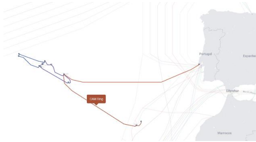
Figure 2. Cable system connecting Azores and Madeira to the mainland. Source: Submarine cable map
