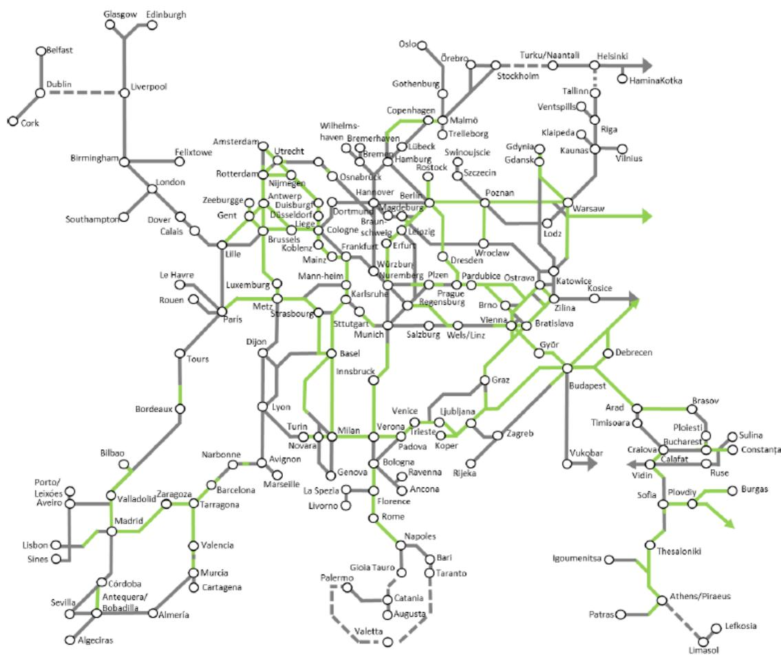
*ERTMS operational lines (either passenger or freight) shown in green on the schematic map of the Core Network Corridors.*
