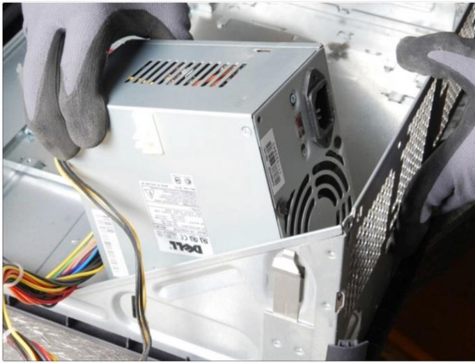
Fig. 7: Removal of the Power Supply Unit
