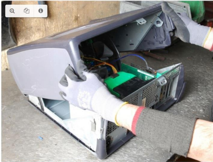
Fig. 5: Disassembly of the PC casing
