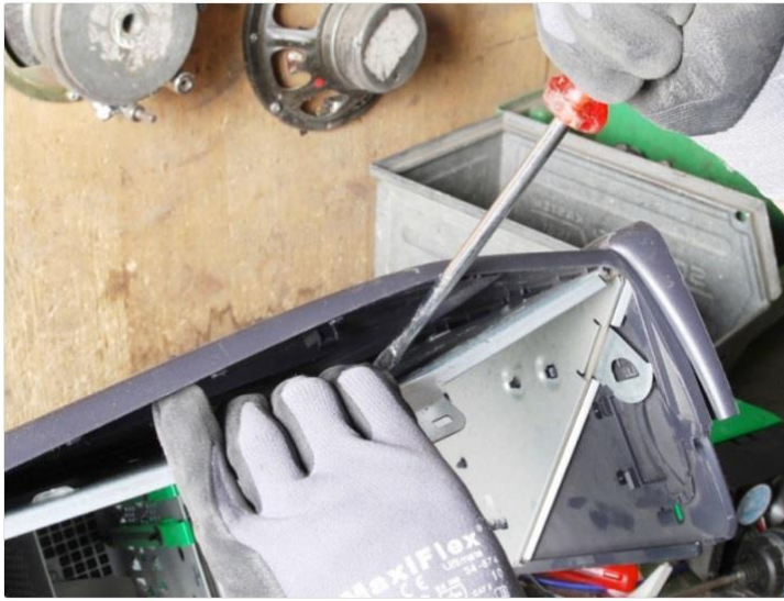
Fig. 9: Separation of the residual parts from the PC casing
