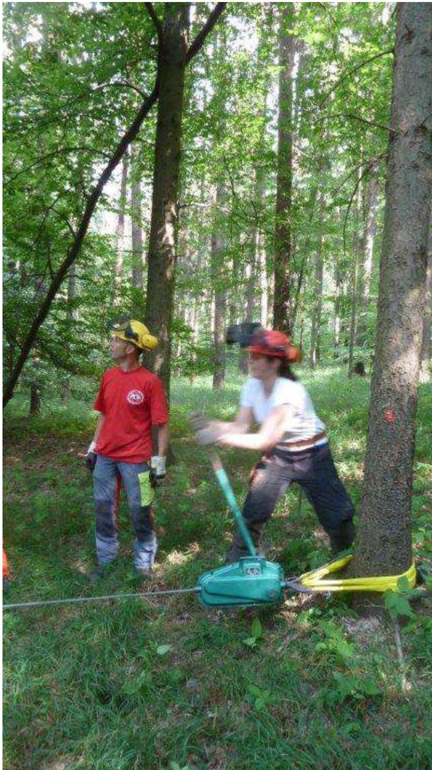
(Photo 13: ICC2 Taking down a hung-up tree with a hand-winch –Czech Republic: Robb 2011)
