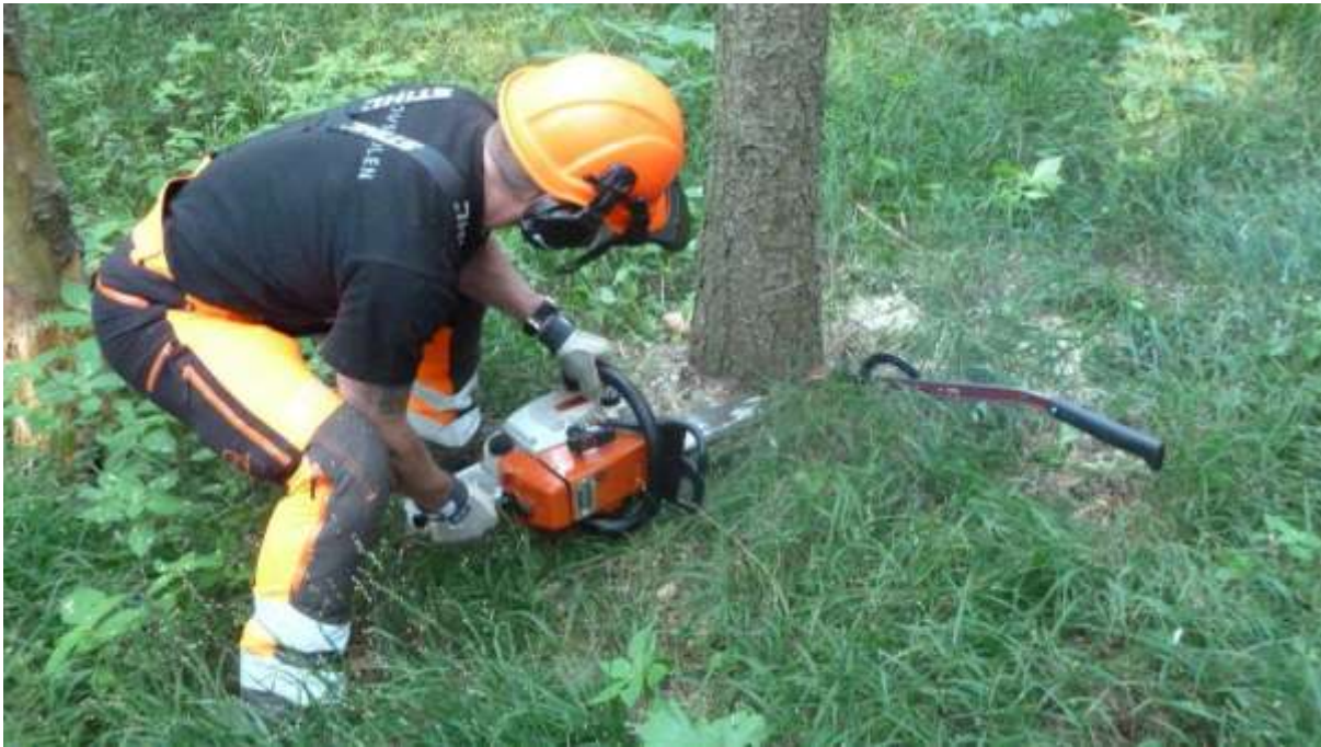
(Photo 7: ICC2 Demonstration of the Danish felling method-Czech Republic: Robb 2011)
