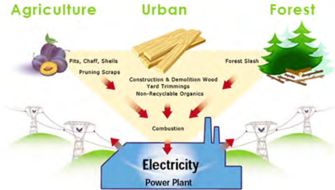
Figure 10.5. Sources of biomass for power generation ( http://www.calbiomass.org/wp-content/uploads/2013/02/biomass-fuel-sources.jpg )
