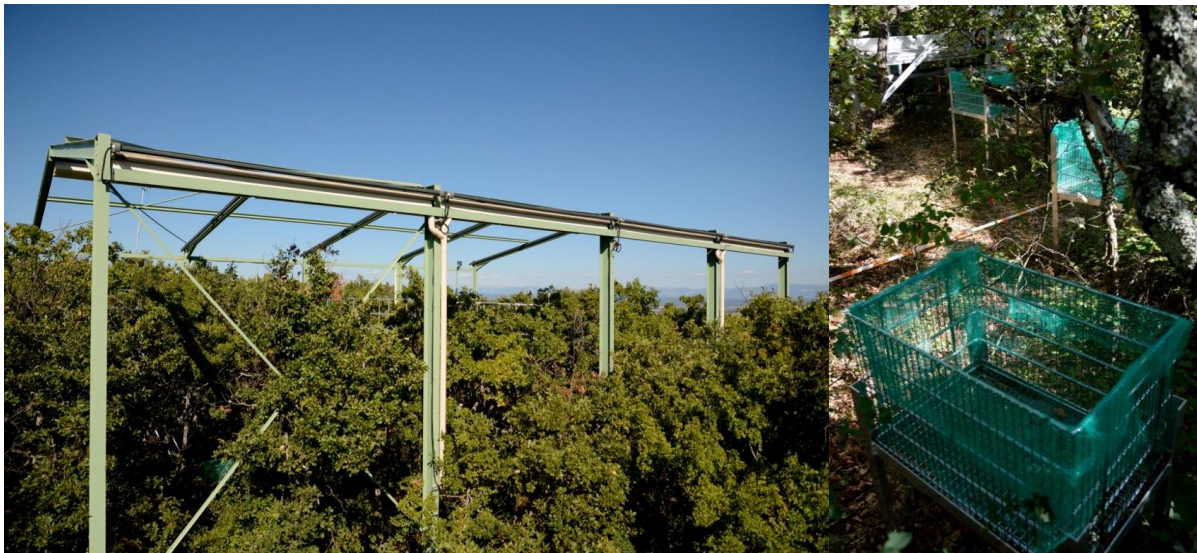
Fig. 2 + 3: The rainfall manipulation experimental device. When it starts raining, the roof can be closed and this will exclude the water for the trees under the roof. There are also several different measurements done under the canopy of the manipulation experiment, like litter fall gathering or litter decomposition experiments.
