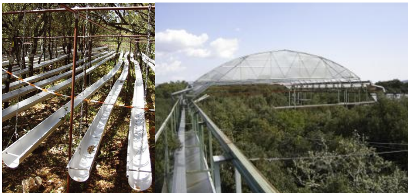
Fig. 2 : Rain-fall exclusion systems of Puechabon. Gutters (left, 30% exclusion) and a dynamic rain-out shelter (right, 100% summer-drought)
