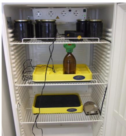
Fig 1: Brown glass bottles with sample Fig 2: Thermostated oven ( 20^\circ \text{C} ) (BOD cabinet)
