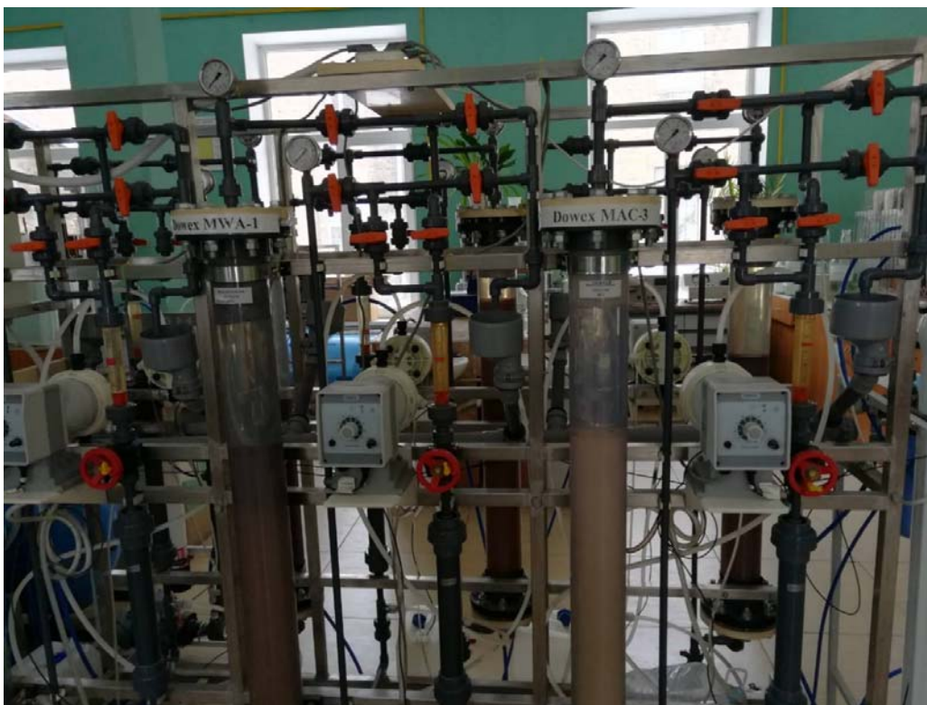
Figure 2: The photo of installation for the determination of dynamic exchange capacity of cation exchanger
