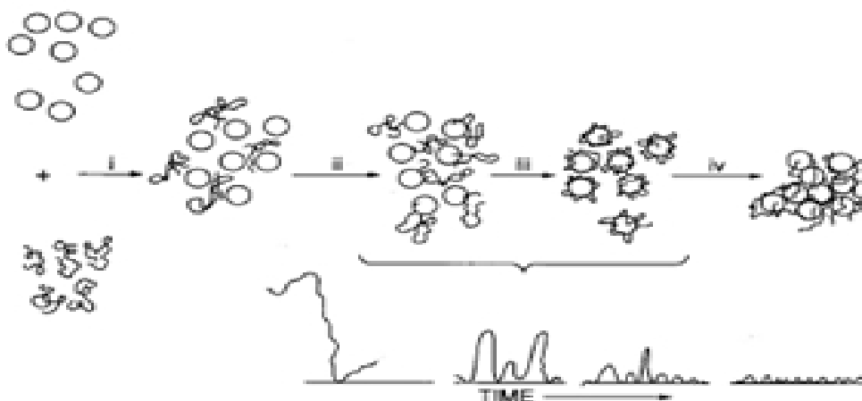
Figure 2: Stages in the bridging mechanism: (i) Dispersion; (ii) Adsorption; (iii) Compression or settling down (see inset); (iv) Collision
