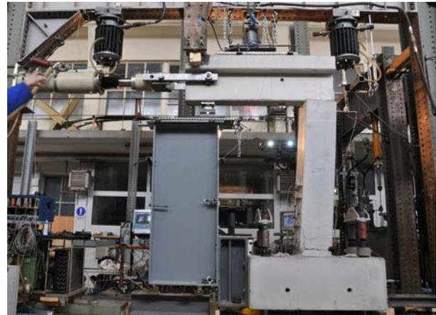
**Figure 9:** Beam-to-column joint
