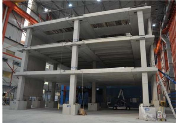
**Figure 11:** Three storey prototype completed
