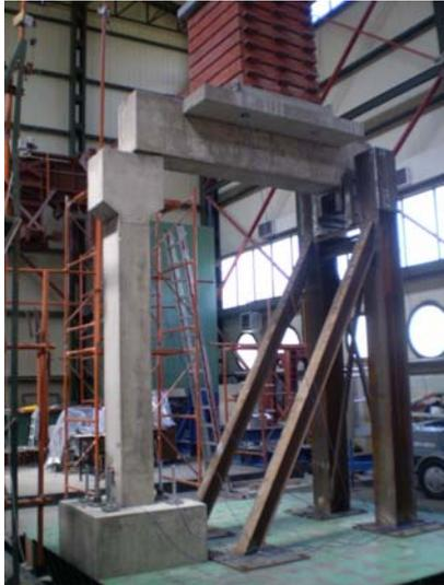
**Figure 5:** Beam-to-column joint
