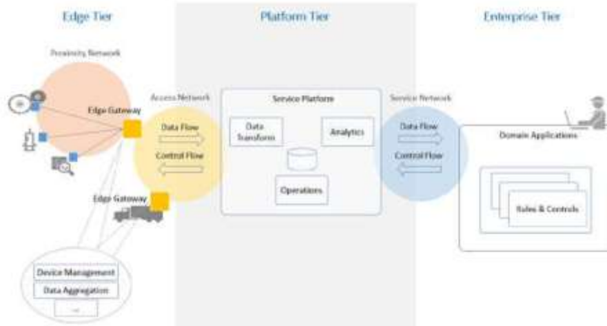
Figure 9: IIC three tier IIS architecture
