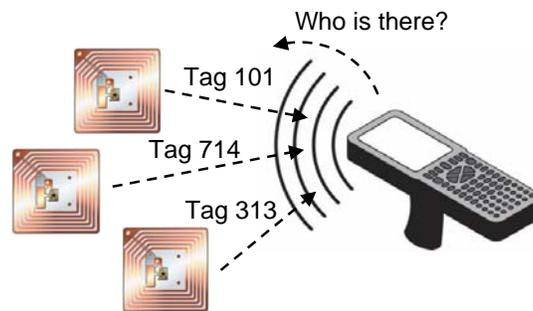
Figure 4. A tag singulation example
