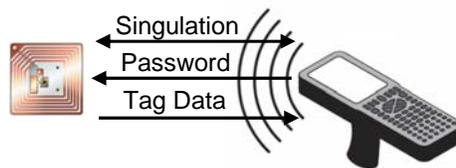
Figure 9. Password-protected tag content access
