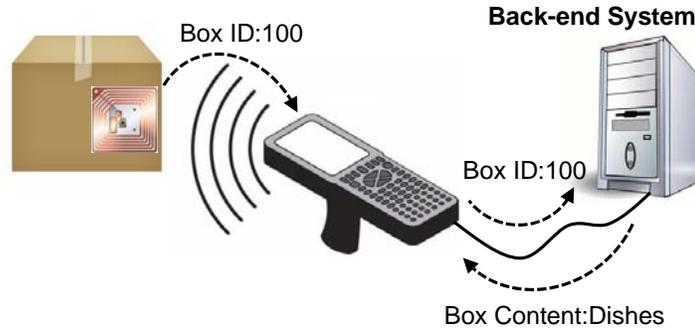
**Figure 2. Typical scheme for RFID tags used for item labeling**
