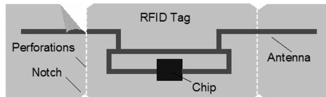
Figure 10. Tag with partial antenna removal (figure credit: [23])
