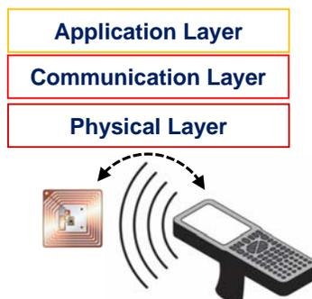
**Figure 3. Tag-Reader communication architecture**
