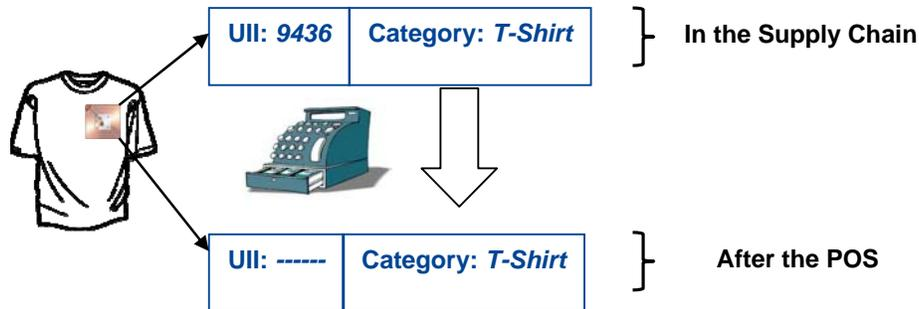
Figure 8. Example of tag data modification at the POS for reducing the tag traceability
