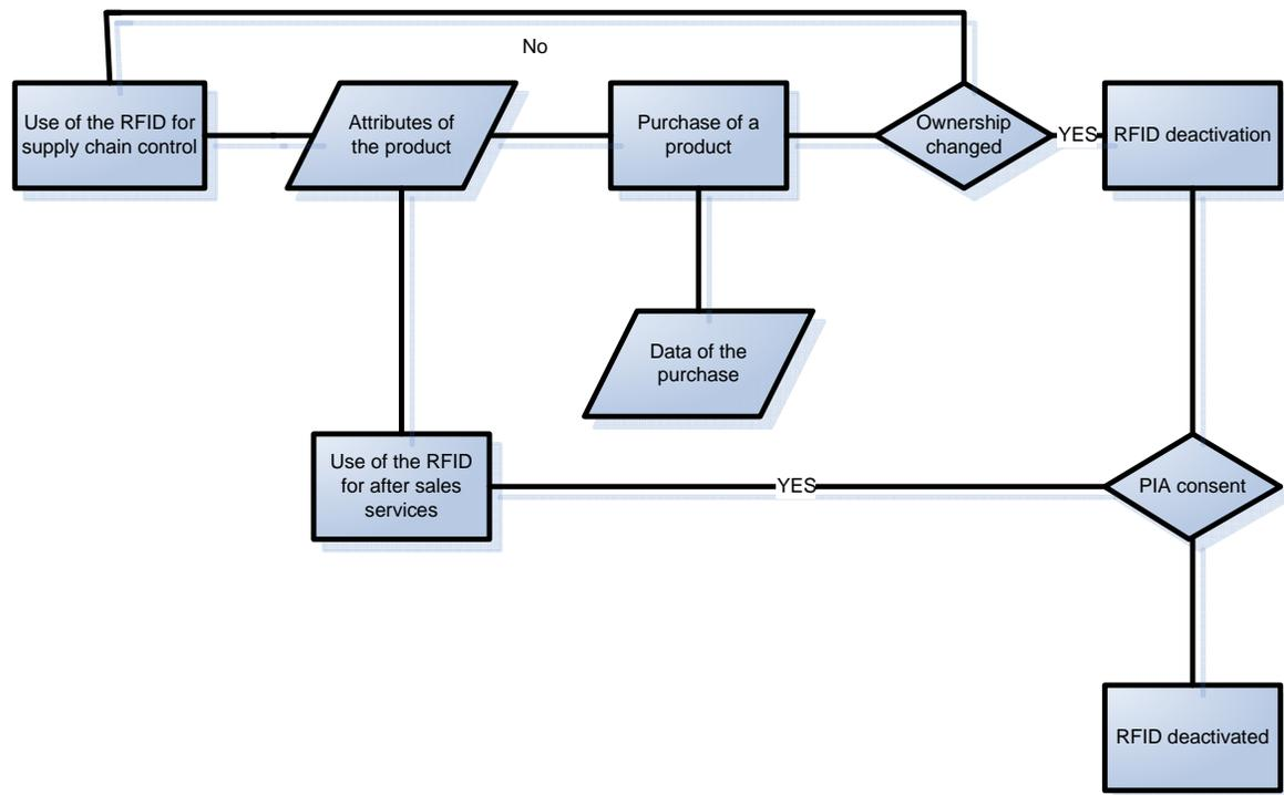
**Figure 13. Flowchart of the process at the POS relevant for the RFID**
