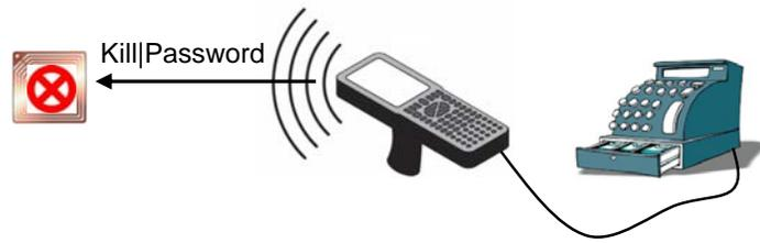
**Figure 11. Kill command applied at the POS**
