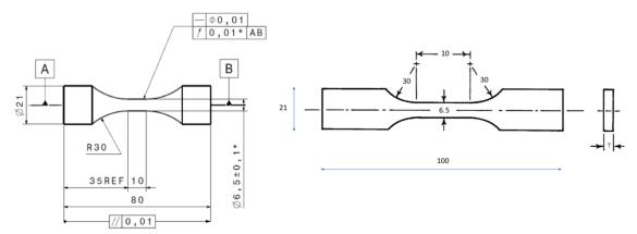
Figure 1: Fatigue test specimen design and dimensions
