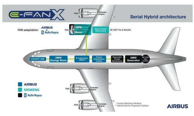
*Figure 2. Main features of the E-Fan-X hybrid electric system layout.*
