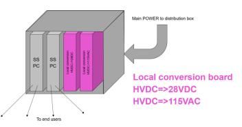
The main technical challenge of this call is to design and develop an High Voltage Direct Current conversion function, in a modular way, to sustain a hot environment with limited cooling capabilities (only passive).
