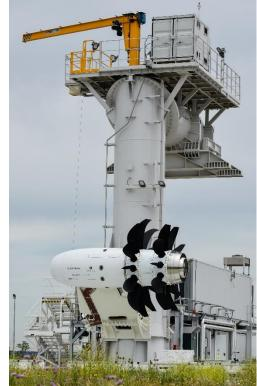
Figure 1. Engine test in Clean Sky
