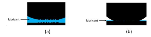
Pictorial representation of solid material contact with full lubrication (a) and boundary/starved lubrication (b). Condition (b) may lead to material scoring/damage.
