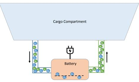
Figure 1: Schematic representation of the envisaged inertisation concept
