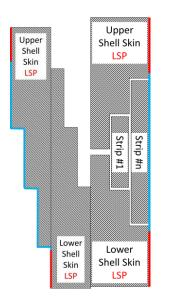
Figure 4: A CFRP fuselage requires protection from lighting strike. Therefore, Upper and Lower Shell skins are equipped with a metallic Lightning Strike Protection. Electrical continuity must be achieved across the longitudinal joints on the outside of the fuselage. Left: Overlap Joint. Right: Butt Strap joint. Red indicates pre-equipped Lightning Strike protection, blue indicates Lightning Strike Protection to be applied as part of this topic.
