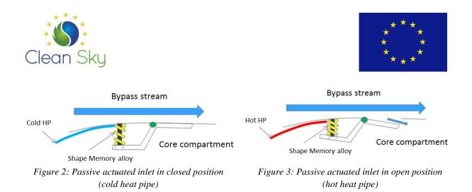
The second part consists of a heat pipe connected to the memory shaped spring, acting as a passive measurement mean. Indeed, the heat pipe can be placed in very strategic and sensitive areas of the engine core zone and will enable the control of the memory shaped spring using the temperature level of a sensitive area distant from the ventilation inlet.
