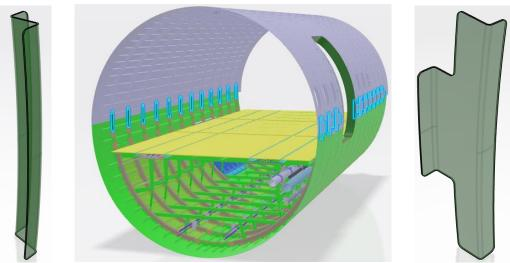
Figure 5: Frame coupling integration: Frame couplings differ per side.
