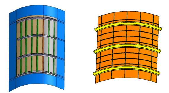
Figure 2: 3D model of the fuselage panels to be manufactured and tested (metallic left and TP right)
