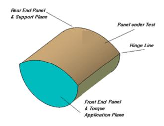
Figure 4: Schematic of D-Box fixture configuration
