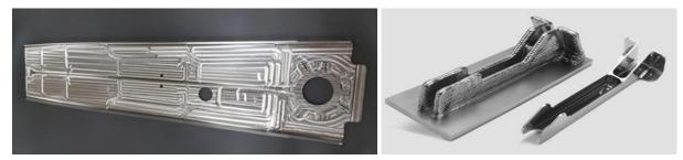
Figure 2. (LEFT) Study case for Airbus upper rear spar component in Ti6Al4V printed using Sciaky W-DED EBAM [1]. (RIGHT) First FAA-certified Ti6Al4V Structural component galley bracket for Boeing 787 Dreamliner printed using Norsk Titanium W-DED WAAM [2].
