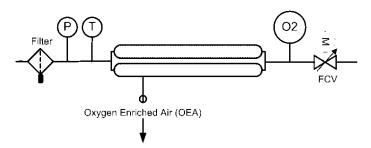
The electrically driven valve shall adjust its passage's section to regulate the flow thanks to electrical current provided to the valve (closed loop system with gauging and flow evaluation means).
