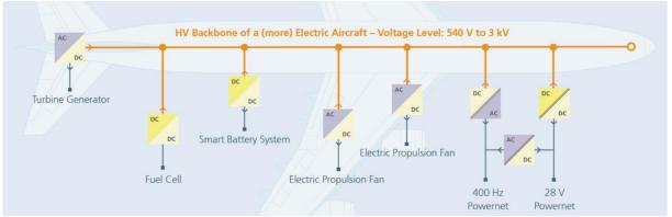
Figure 1: Exemplary energy transmission with distributed electrical systems in a hybrid/electric aircraft system.
