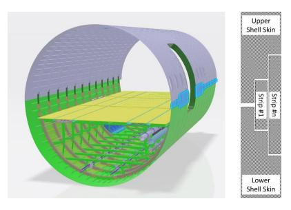
Figure 3: Butt strap integration: A number of overlying strips require integration across the stepped joint. Note that the Butt strap sits on the outside of the fuselage.
