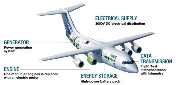
Figure 1. Main features of the E-Fan-X test aircraft.
