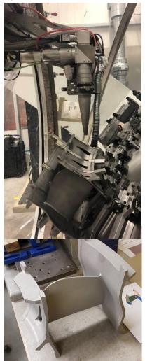
Figure 3. The final demonstrator will probably consist of two super alloy sectors (as above) welded together. Size is typically 25 cm in all dimensions.
