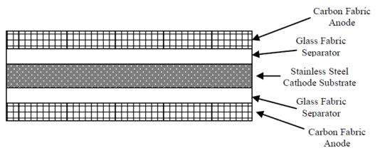
*Figure 2. Example of multifunctional material scheme.*
