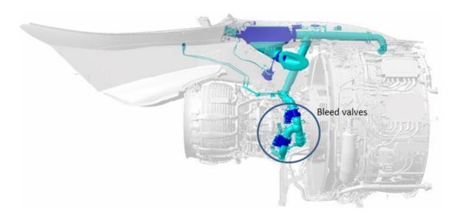
High temperature butterfly valves have to ensure a limited internal leakage in order to avoid pressure build-up in the bleed pipes. To compensate this pressure build-up, pressure relief holes are sometimes necessary in the bleed pipes. The Topic Manager currently uses cobalt alloy like stellite 6 for the manufacturing of the butterfly sealing rings that slide against a hard chromium coating or a tungsten carbide-cobalt coating.
