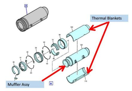
Figure 1 – Typical APU muffler components
