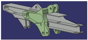
Figure 1:. Flap support concept - roller track and carriage
