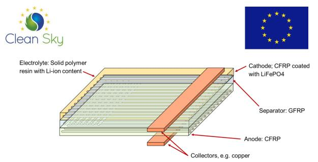
Fig. 3. Multi functional material battery, here a composite battery consisting of anode (CFRP), Separator (GFRP), cathode (CFRP + LiFePO4 coating), copper current collectors.
