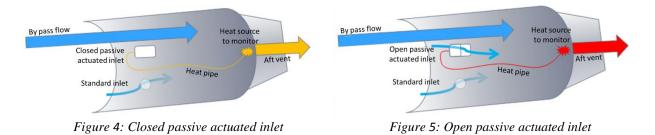
Therefore, the complete system allows the passive modulation of the engine core zone ventilation and, as a consequence, the thermal management of sensitive areas of the engine core zone as close as possible from the cooling needs of these areas.
