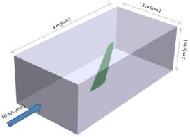
Figure 2 Minimum Wind Tunnel dimensions and speed
