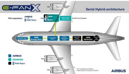
There are currently no large electric or hybrid aerospace power systems in operation, therefore no aerospace insulation monitoring system demonstrators available. Demonstrators, such as E-Fan X (see above Figure) and EcoPulse, are planned by numerous European aerospace companies and while all are likely to require insulation monitoring as a system enabler, few aerospace companies have significant experience with creating insulation monitoring systems.
