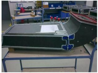
Figure 4 Example of Air intake ducting
