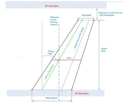
Figure 1 Planform definition of a trapezoizal lifting surface and wind tunnel constraints
