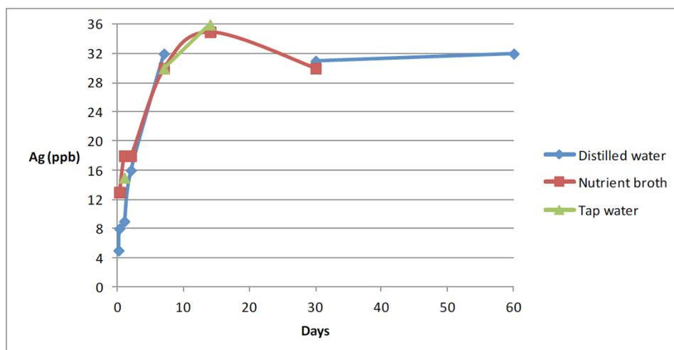
It can be seen from the results of this study that the kinetics of silver migration were comparable for the three simulants investigated. Maximal silver concentrations (~ 35 ppb) were seen up to approximately Day 14. Silver levels subsequently remained relatively constant at a level of approximately 32 ppb. Ref. Taiki 2012
