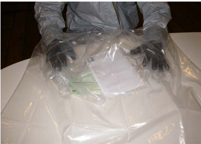
Glove bag for reduction of aerosol dispersal
