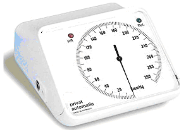
Figure 2 Example of an auscultatory sphygmomanometer, which indicates Korotkov sounds by a flashing LED (red LED on the left). The cuff with the microphone is not shown 3 .
