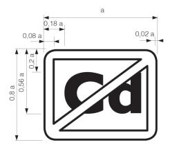
The dimension of "a" shall be greater than 9 mm and the typeface to be used is 'Gill Sans'.
