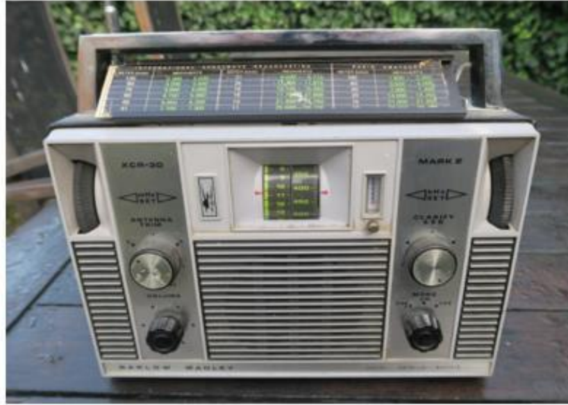
1977 Portable Radio. 18 discrete transistors - count them!
