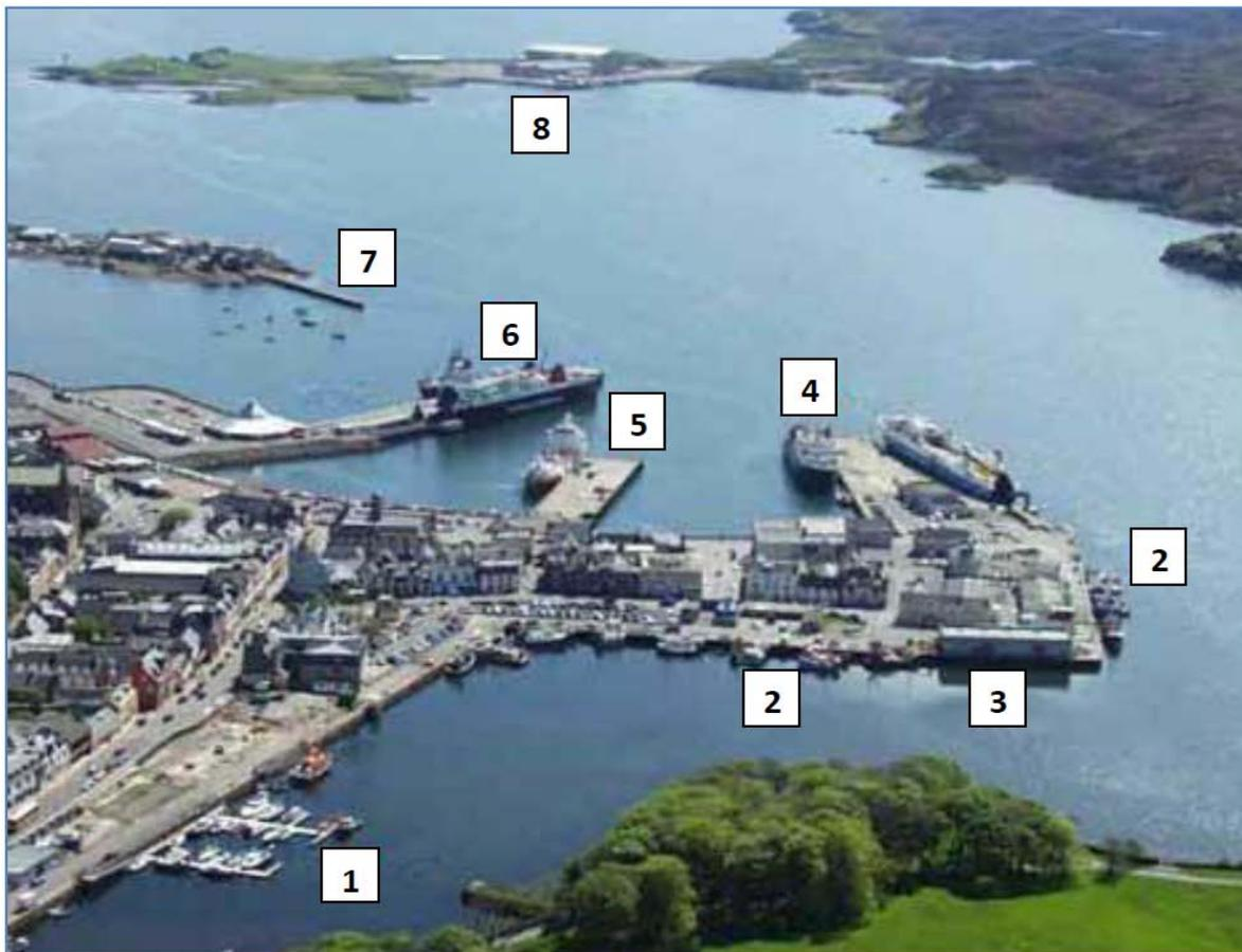
Pontoons for pleasure craft (1), fishing vessel berths (2), fish market and ice plant (3), piers for tankers, freight vessels and visiting vessels (4 and 5), Ro/Ro ferry pier (6), slipway and boatyard (7), and Arnish pier (8).
