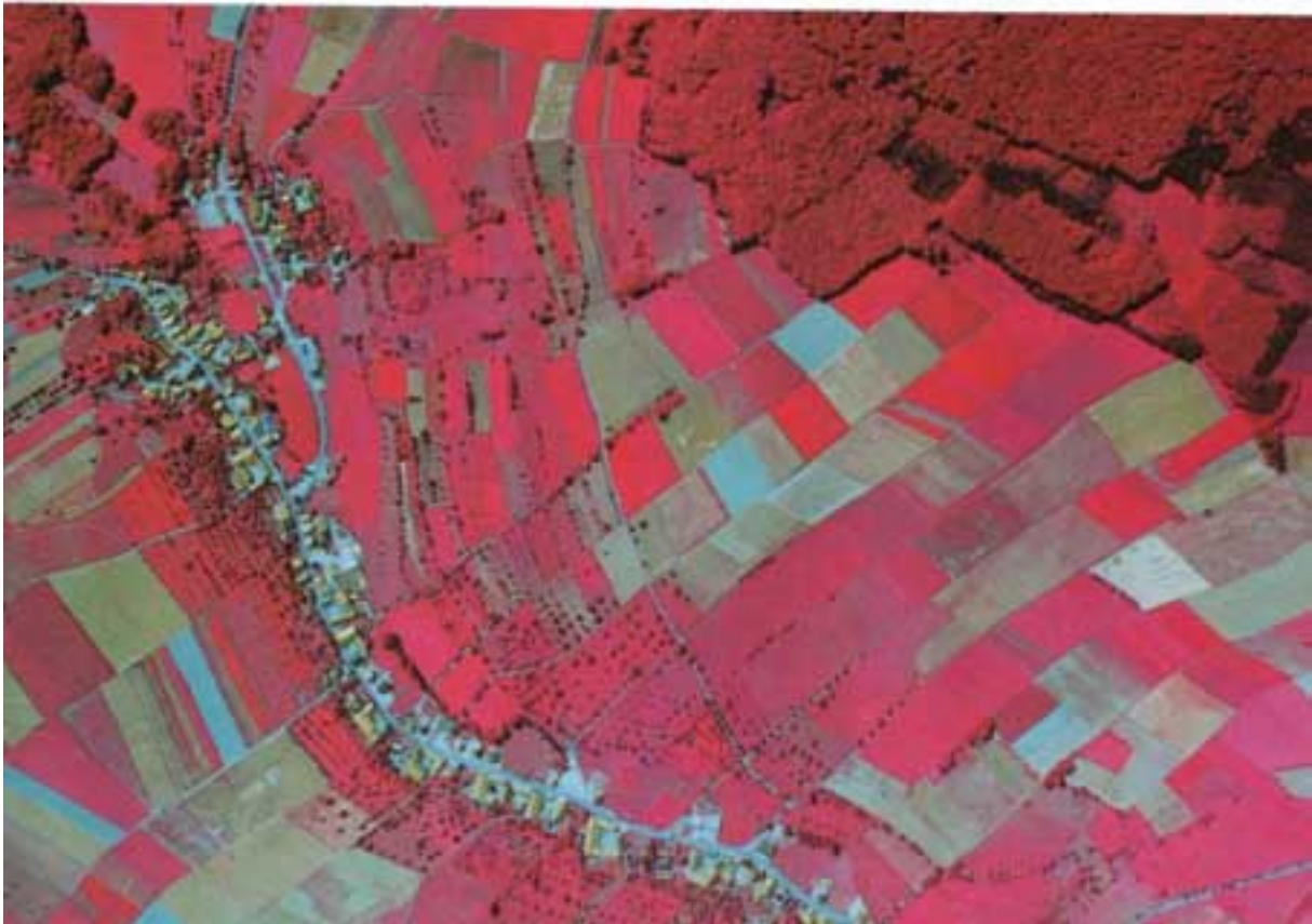
Figure 4.10: Example of a colour and a CIR aerial photography, Odenwald, Germany, date 30.7.67, original scale 1:14.000 (ALBERTZ 1991)
