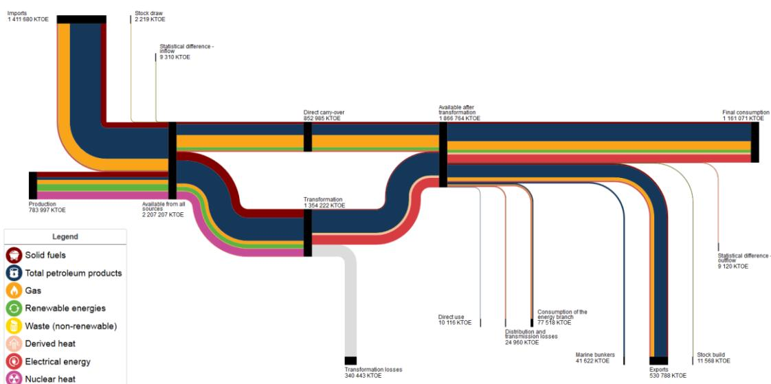
If you look at the Sankey diagram, you can see that most of the energy available in the EU is imported, while only a smaller proportion is produced internally. In the example, around 36% of the energy comes from the Production flow, against 64% which is imported. The most of the energy available is in the form of total petroleum products (including crude oil), followed by natural gas, solid fuels, renewable energies and nuclear heat.
