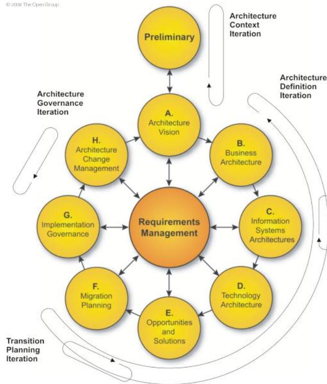
**Figure 2: The Architecture Development Method of TOGAF (The Open Group 2009)**
