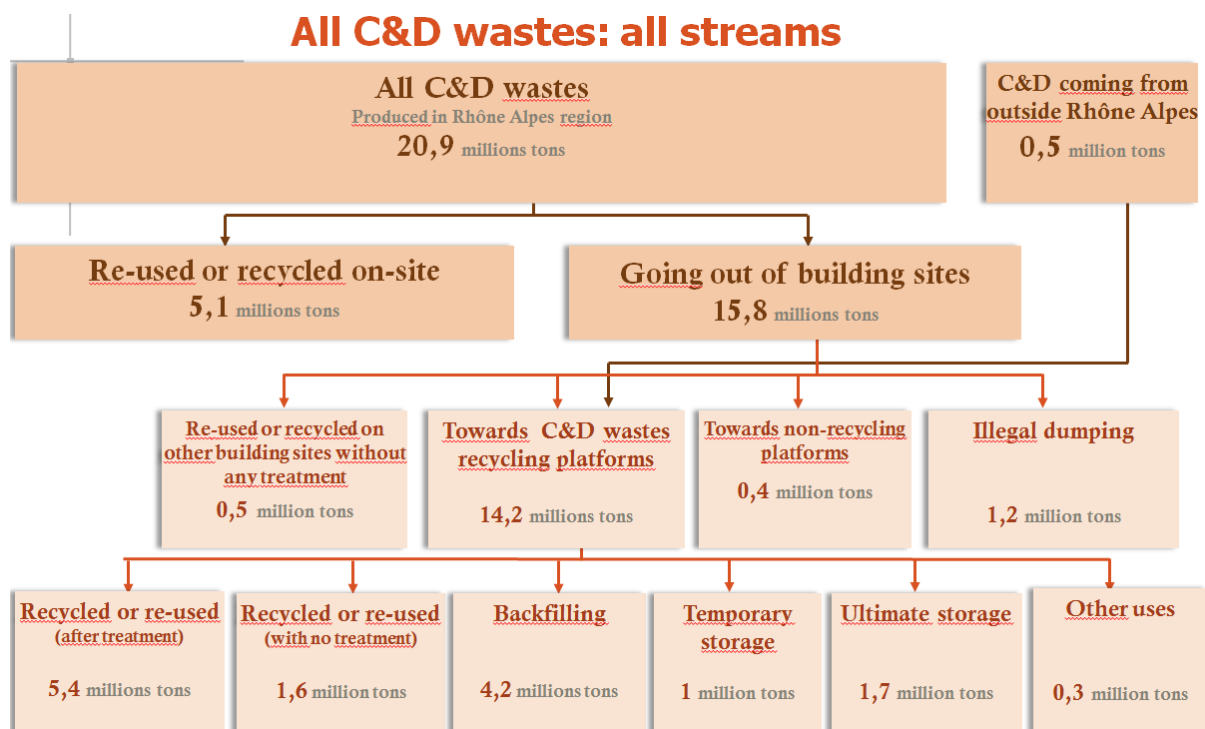
Annex 2: Extract of the study run by the Rhône-Alpes Economic Cell (CERA) on 2012 CDW treated quantities
