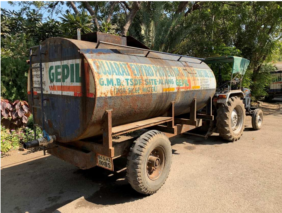
GEPIL tank truck for liquids (bilge, ballast water, oily water, storm water)
