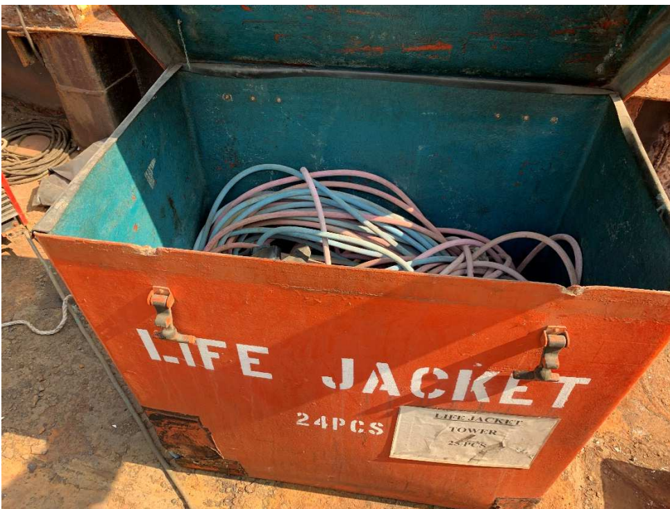
The regime for safety equipment onboard the crane barge needs to be reviewed and actions taken. For example, a container on the crane barge deck was identified as containing lifejackets but when opened was found to contain cables and hoses.
