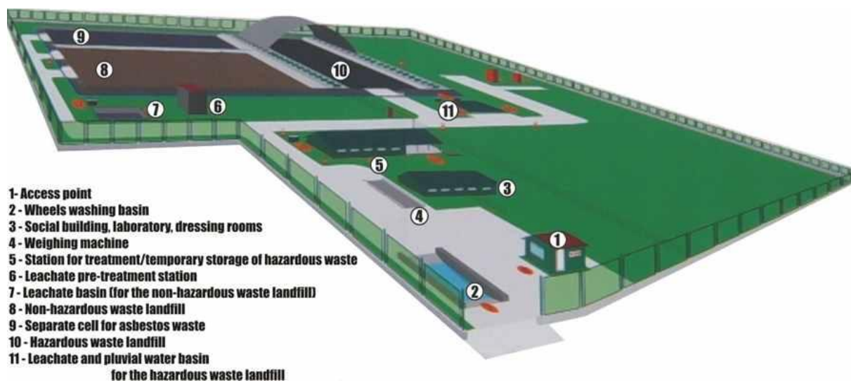
Figure 1.10-1: Overview of the hazardous and non-hazardous landfill sites of Vivani Salubritate S.A. (Romania)
