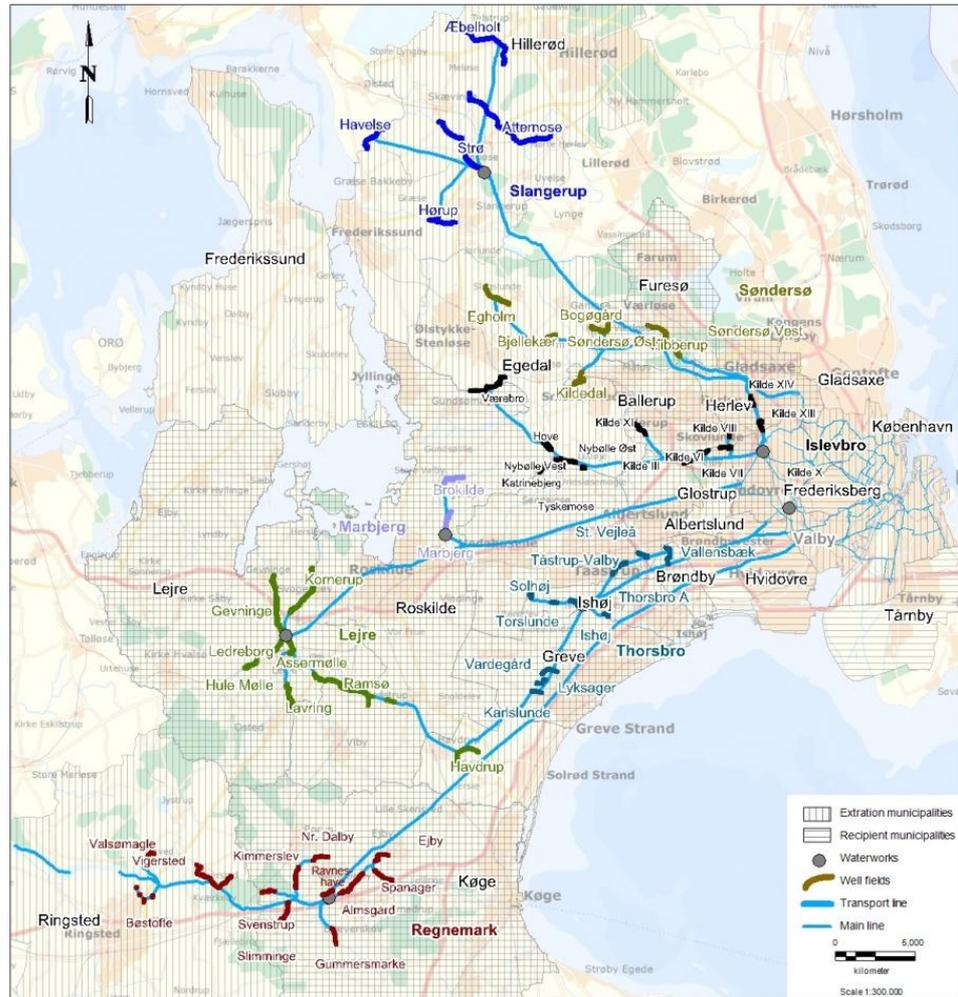
Figure 1. The complex catchment and supply structure of the City of Copenhagen.
