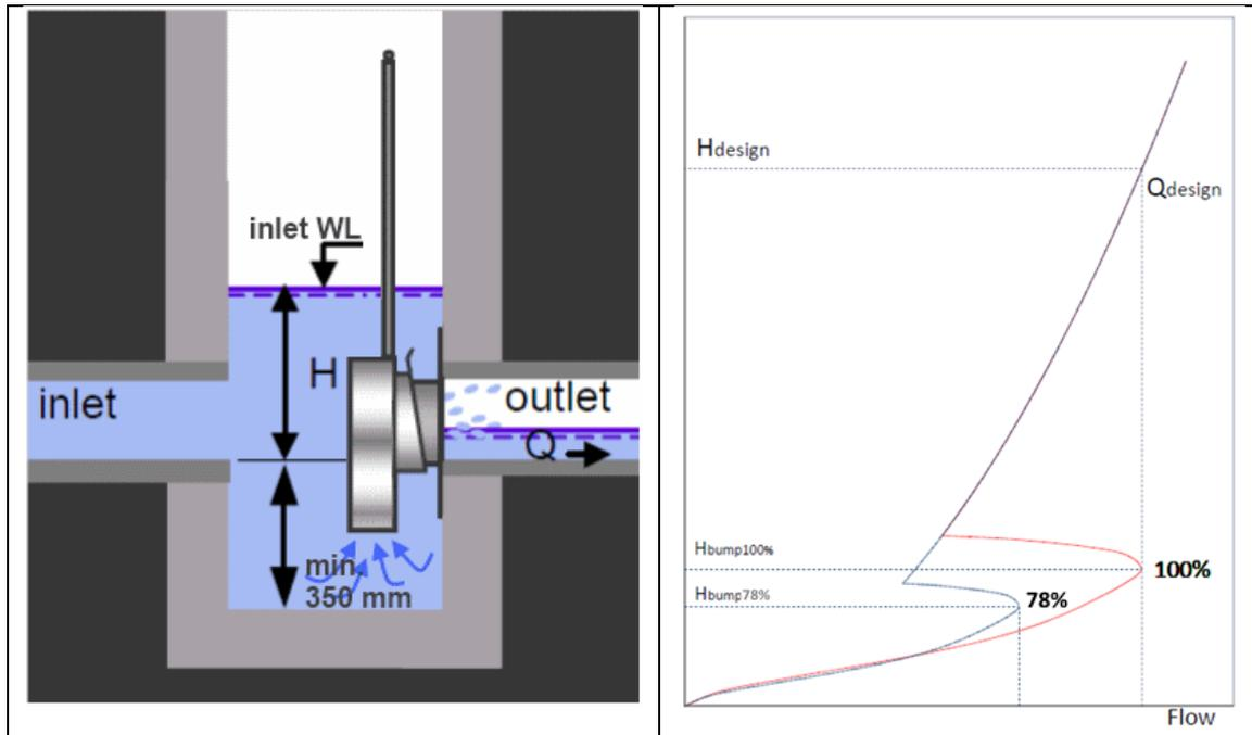
Figure 1 A) Sketch of CEV flow regulator installed in a well.
