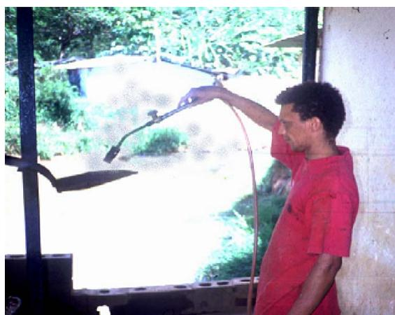
*A miner evaporates mercury from the gold-mercury amalgam with a blow-torch.*
