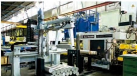
Superconductor technology enables significant energy savings in metal billet heating
