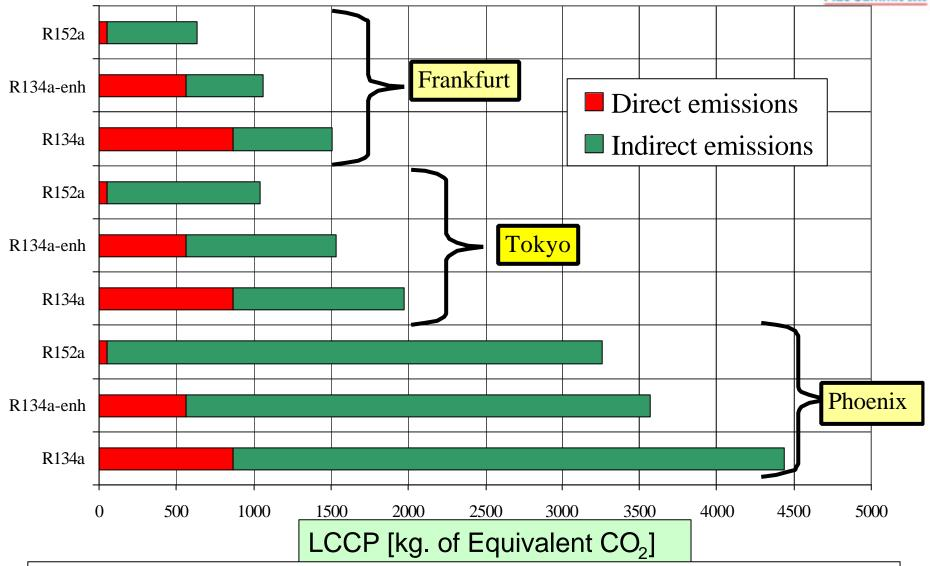
Direct Evaporation System reported by Delphi/GM/EPA at SAE Phoenix Alternate Refrigerant Symposium 2002
