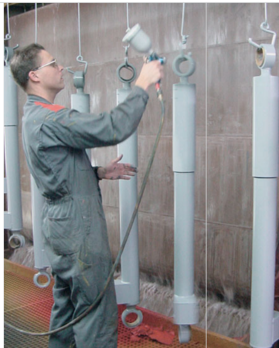
Shock absorbers undergo a series of operations along the full length of a 420 m line.
