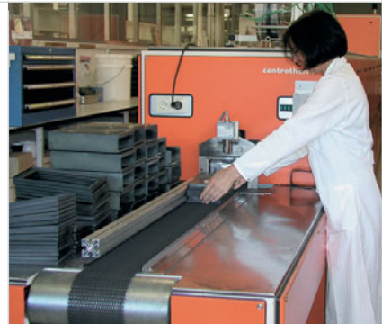
Loading carbon forms into the prototype oven (3 000 diodes per mould).
