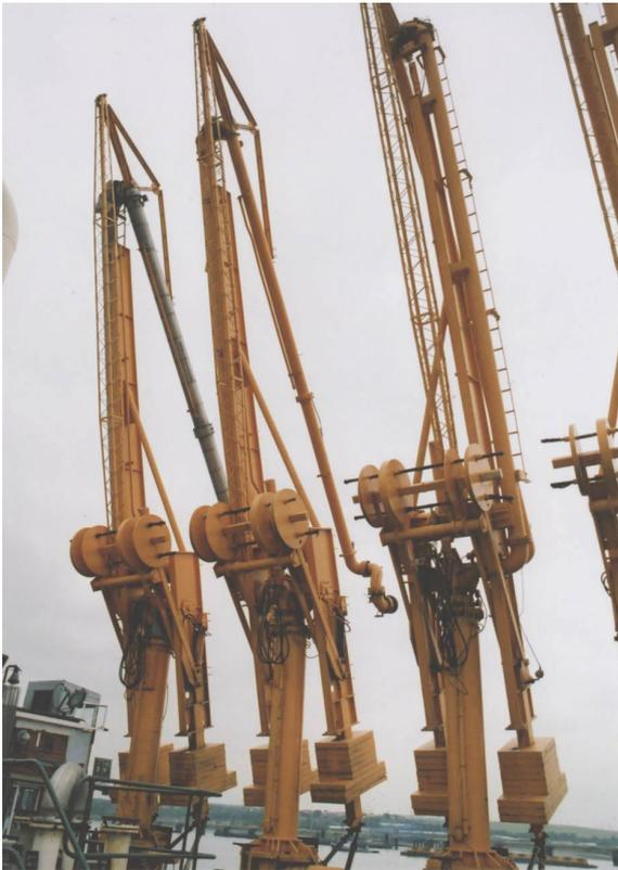
**Figure 9 - Loading arms with vapour return facility**
