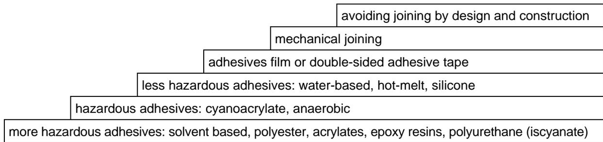
Figure 3-13: Bonding with levels of hazards [Soerensen 1998]
