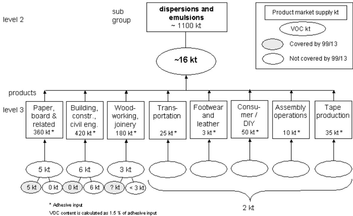
Figure 2-24: Adhesive and VOC input for dispersions and emulsions in industry sectors in Europe [Derived from PRODCOM and UBA/VCI 1997]
