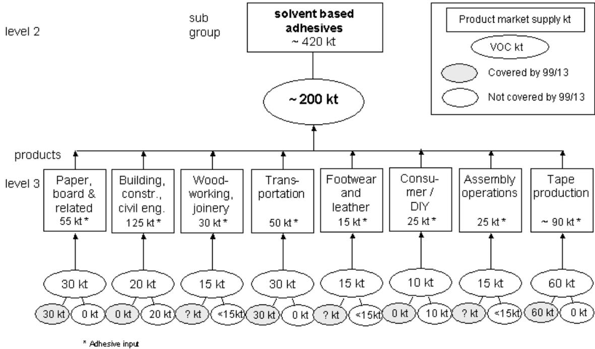
Figure 2-23: Adhesive and VOC input for solvent based adhesives in industry sectors in Europe [Derived from PRODCOM and UBA/VCI 1997]
