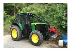
RDP support was used to acquire a four-wheel drive standard tractor designed exclusively for forestry work and other necessary equipment, such as nets and safety equipment, a forestry winch and a pulley.
