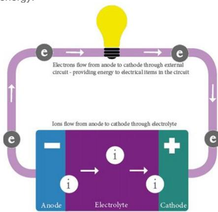
**Figure 3. Schematic overview of the functioning of an average battery.**
