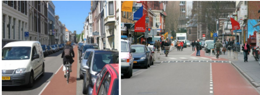
Contra-flow cycling with advisory lane or cycle lane, in narrow and wide one-way streets (image source: D. Dufour, P. Kroeze)
