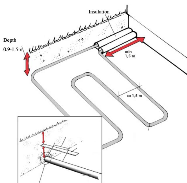
**Figure 2 Example of ground coil configuration**
