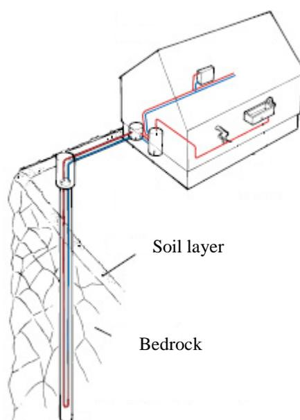
**Figure 4 Vertical ground rock collector**
