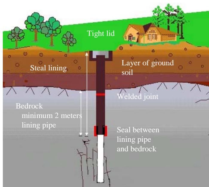
**Figure 5 Configuration in compliance with Normbrunn 97**
