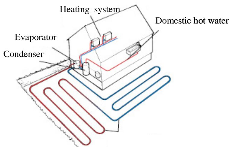
**Figure 1 Indirect ground soil system**
