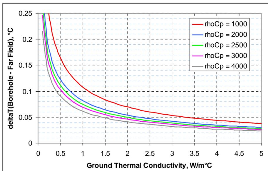
Figure 3.1 Temperature reaction of a borehole
