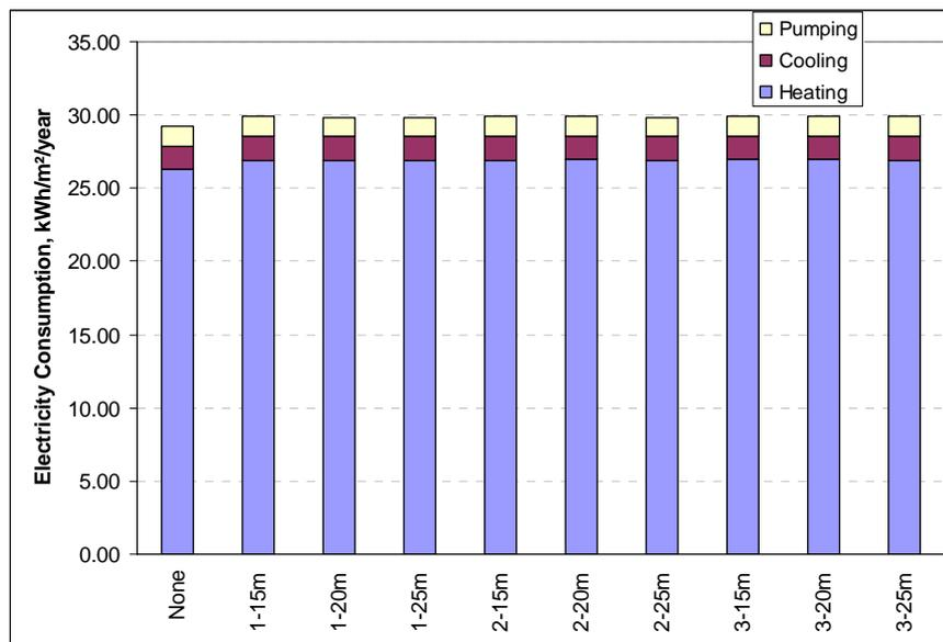
Figure 6.1 Electricity consumption of heat pump systems with neighbors
