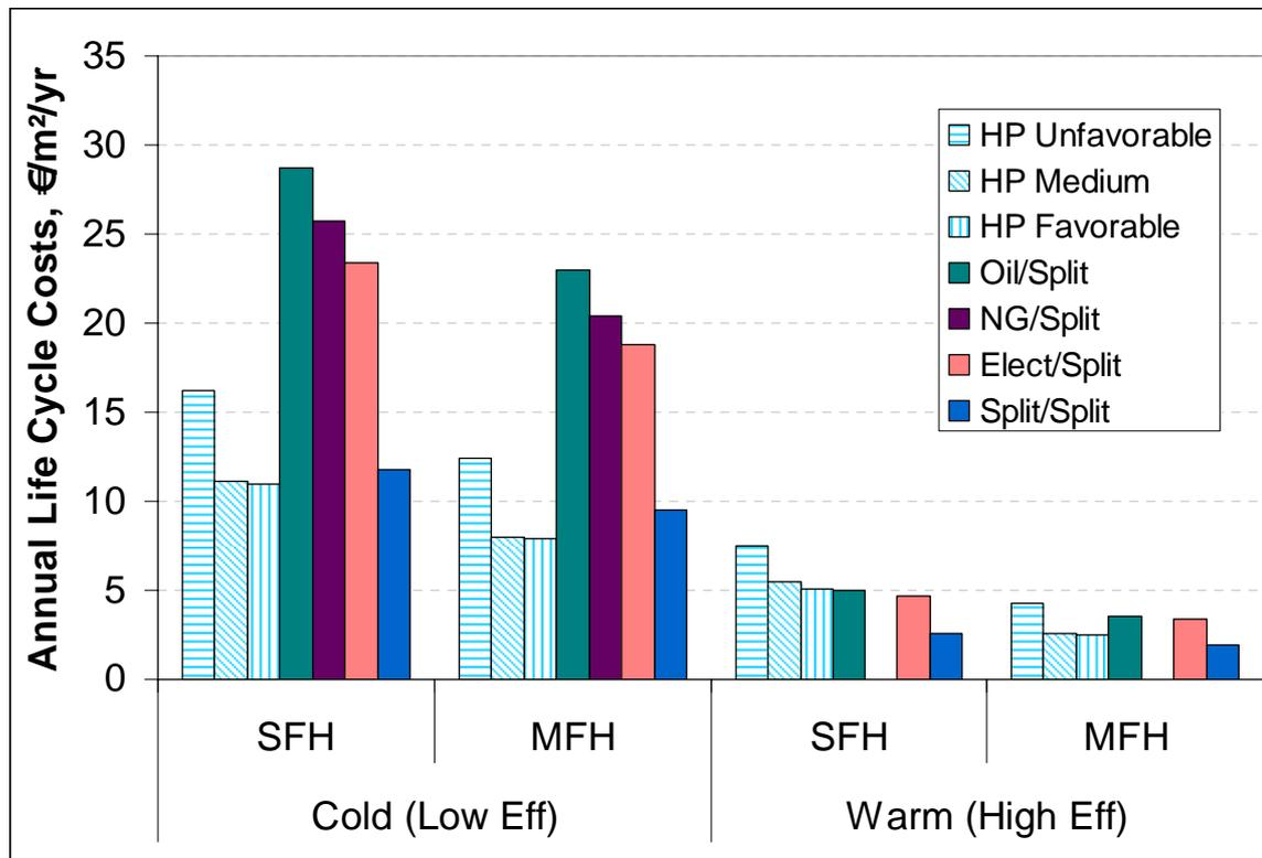
Figure 3.3 Life cycle costs of heat pump and alternative systems for different ground properties
