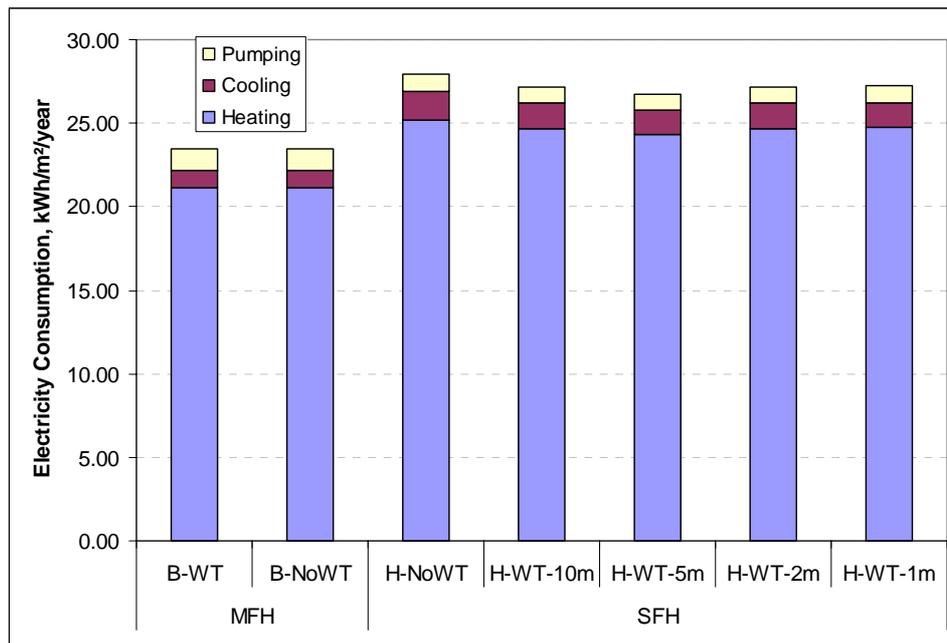
Figure 5.2 Energy consumption of GCHP systems with aquifers
