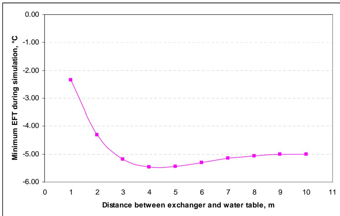
Figure 5.1 Minimum EWT as a function of water table location
