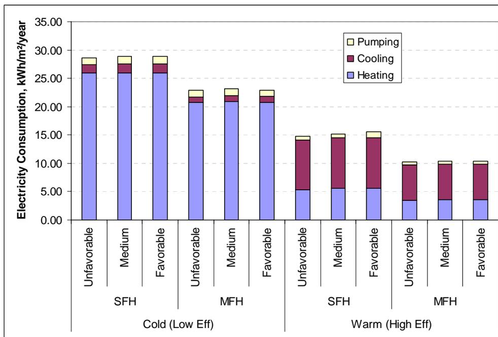
Figure 3.2 Heat pump systems electricity consumption for different grounds.
